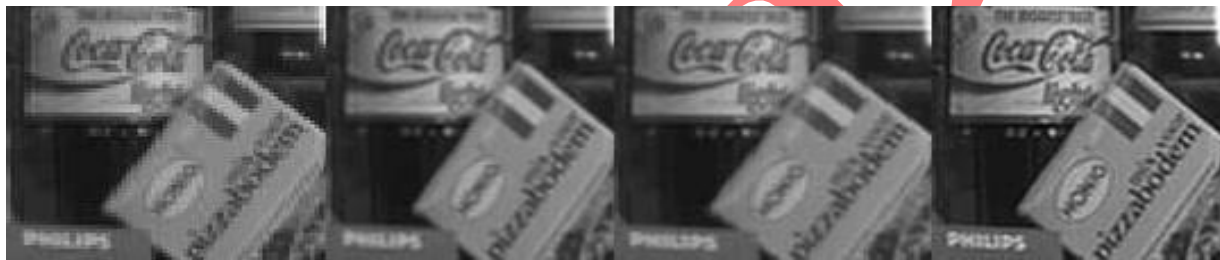
Figure 2.3: POCS SR results (a) by bilinear interpolation and by POCS after (b) 10 iterations, (c) 30 iterations, (d) 50 iterations [2].
